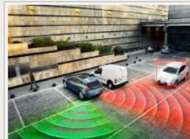
An illustration shows how a cross-traffic alert system works, by spotting oncoming traffic.
