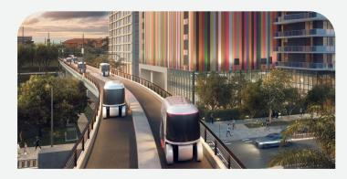
Smaller Right of Way 5.5'-15' Wide guideways (single/double) Scalable Capacity
